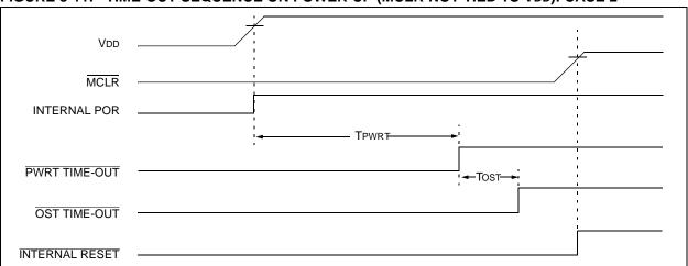
FIGURE 8-12: TIME-OUT SEQUENCE ON POWER-UP (MCLR TIED TO VDD): FAST VDD RISE TIME
