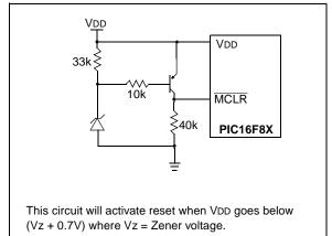
FIGURE 8-15: BROWN-OUT PROTECTION CIRCUIT 2
