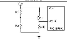
This brown-out circuit is less expensive, although less accurate. Transistor Q1 turns off when VDD is below a certain level such that:
