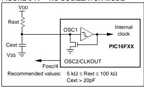
**Note:** When the device oscillator is in RC mode, do not drive the OSC1 pin with an external clock or you may damage the device.
